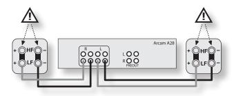
An A28 connected to speakers using single wiring
